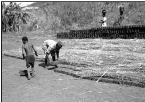
Above: Laying the molded bricks out to dry. They're going to need a lot of room for 300,000 more!
